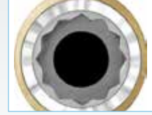
The 12-point double hex, which is machined in the 15° Pre-Angled GingiHue Abutment, provides rotational positioning in 30° increments on the implant hex.
