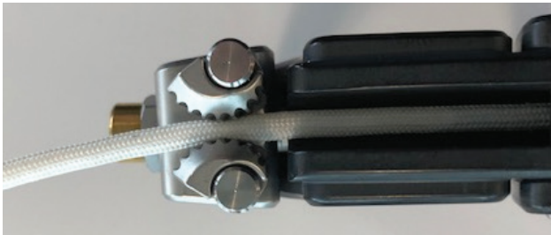
Figure 25 Tensioner rack and cleat capture of cord
